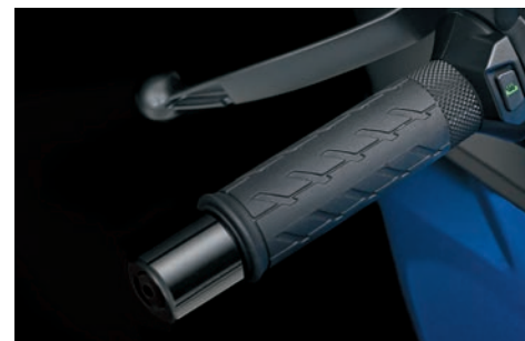
Grip heater 57100-48821 With three different heat settings. *Entire surface is heated
