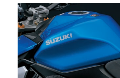
Fuel tank protection foil (Transparent) 99181-48K00 Protects against tank scratches.
